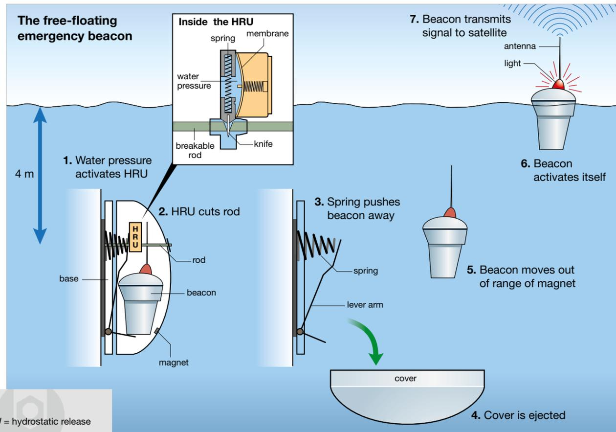
HRU = hydrostatic release unit
